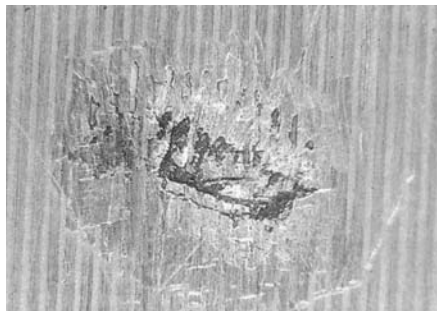
Surface fatigue on ball bearing
